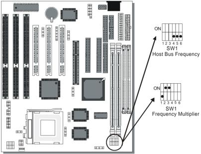
The SY-5EHM/5EH5 V1.2 Motherboard is designed to support most Pentium® class processors currently on the market. Jumpers SW1 is used to configure the Motherboard frequency parameters to match the working frequency of your CPU.
